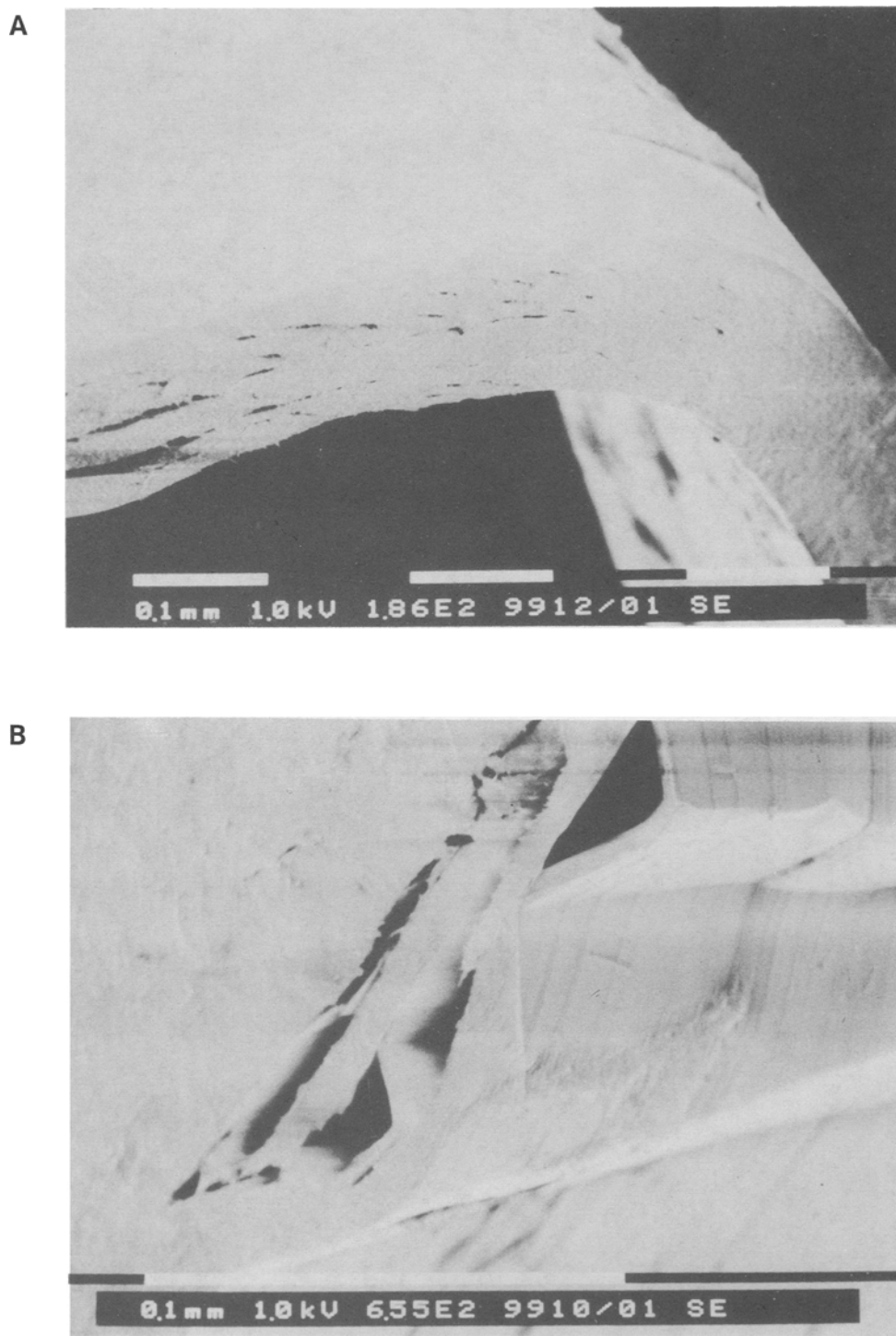
FIG. 17. Mechanical deformation of \beta' LML crystals. (A) Detail of rupture between layers in an irreversibly bent \beta' crystal. (B) Buckling of crystal layers on the inside of a bent crystal.
